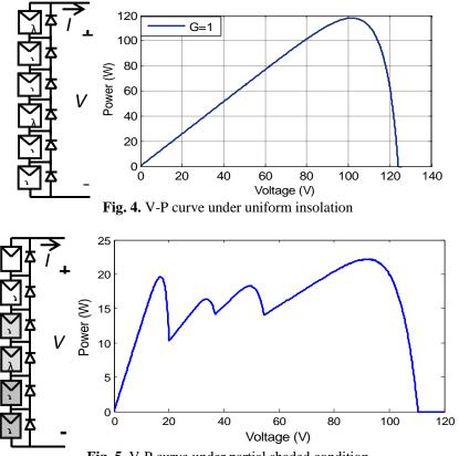
Fig. 5. V-P curve under partial shaded condition
