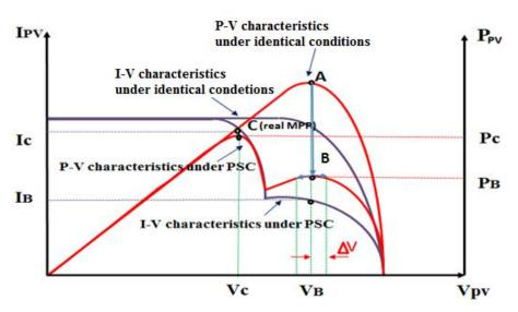
Fig. 6. P-V and V-I characteristics of PV cell under shaded and unshade conditions
