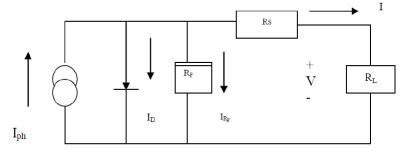
Fig. 1: Equivalent circuit model of PV cell.
